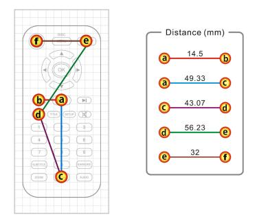
Figure 7. Distance between Buttons and Number of Button Combinations
