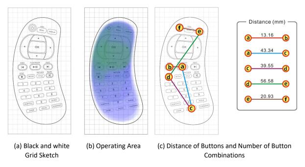
Figure 9. New Design Plan of Remote Control New D
